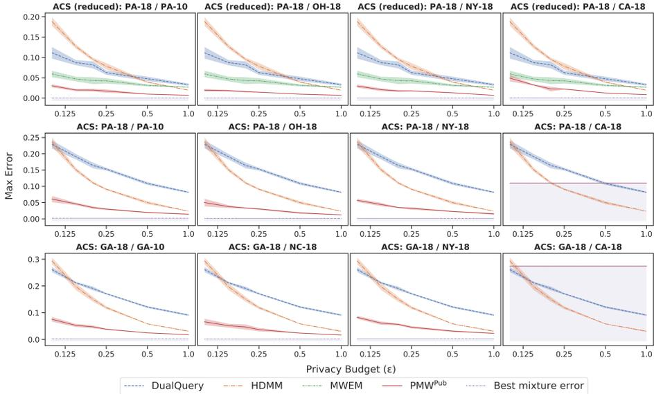
Figure 1: Max error for  $\epsilon \in \{0.1, 0.15, 0.2, 0.25, 0.5, 1\}$  and  $\delta = \frac{1}{n^2}$ . Results are averaged over 5 runs, and error bars represent one standard error. The  $x$ -axis uses a logarithmic scale. We shade the area below the *best mixture error* to represent max error values that are unachievable by  $\text{PMW}^{\text{Pub}}$ .
